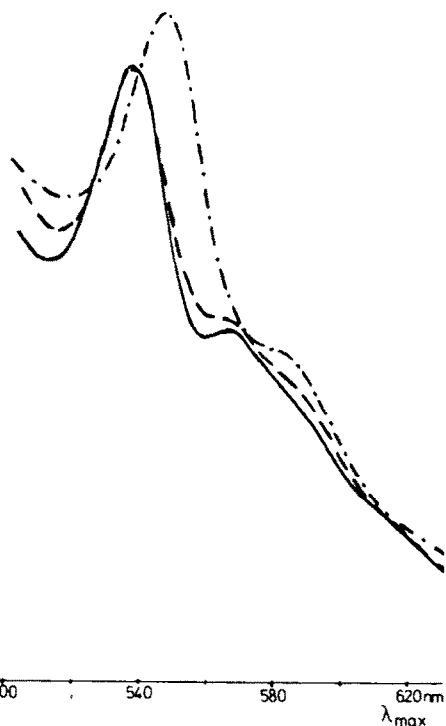
Figure 2. Visible spectrum of 1-methylimidazole-("C 3 -capped porphyrin")iron(II) (24): [ ————— ] under argon [ - - - - - ] under carbon monoxide [ - · - · - ] under argon after two carbonylation-decarbonylation cycles.
